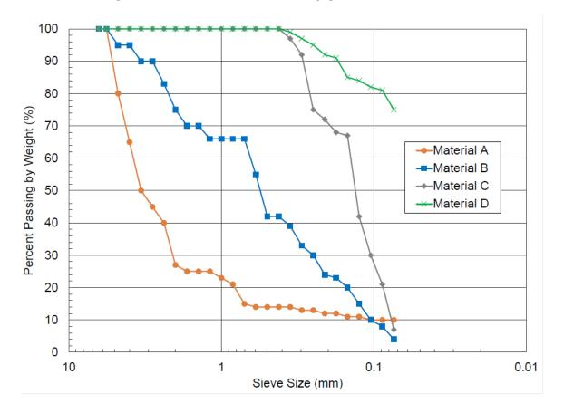
A geologist is evaluating grain-size curves from four potential borrow sources for use in constructing a levee in the Central Valley. The engineer has indicated that the levee will cross a few alluvial deposits of sands and silty sands which will be excavated and replaced with compacted low permeability material to reduce under seepage. Which of the borrow materials is most suitable for use by the engineer designing and constructing the levee?
